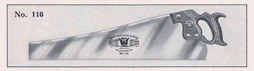
The No. 110 is a popular price Hand Saw made to meet the demand for a medium price, good quality saw. It is made from Crucible Steel, full width, high polish, skew back, ribbon edge, cherry handle; spindle carved, attached with four brass screws and medallion.
