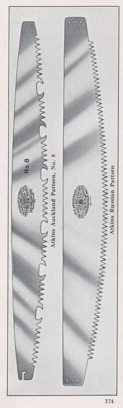
Atkins No. 8 Auckland Pattern. Special Steel. Gauge, 14 x 17. Space of teeth in 6 foot and 6½ foot saws, 1 inch from point to point; in 7 to 10 foot saws, 1¼ inches. Space between sections of teeth, 2 inches.
