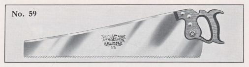
No. 59 is a companion to the No. 58 except it is skew back, made of high quality cast steel fully warranted. The handle is of thoroughly seasoned beech, varnished and polished all over. Fastened to blade with three brass screws and a medallion.
